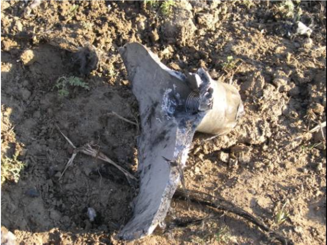
Figure B-13. Portion of Cylinder Found 35 ft From Test Site.
