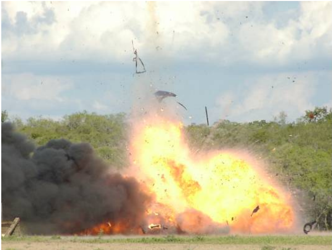
Figure B-7. Explosion of Cylinder, After Approximately 12 Min of Exposure.
