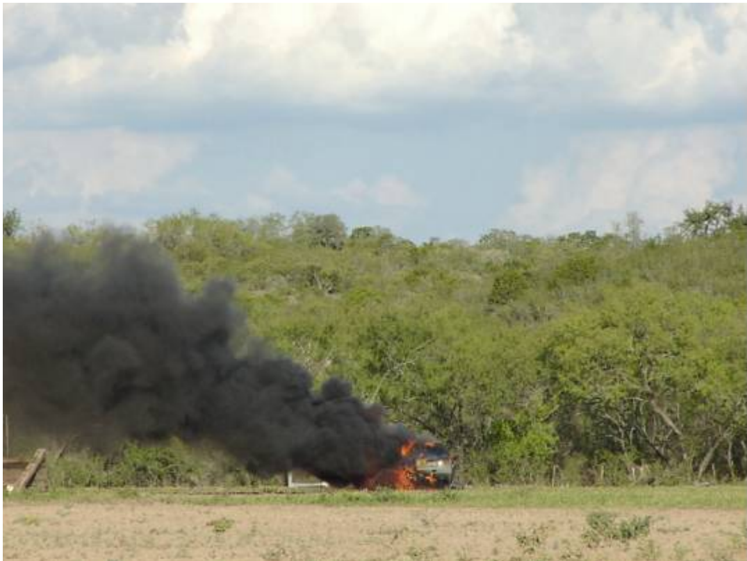
Figure B-6. Full Engulfment of Vehicle, Approximately 10 Min of Exposure.
