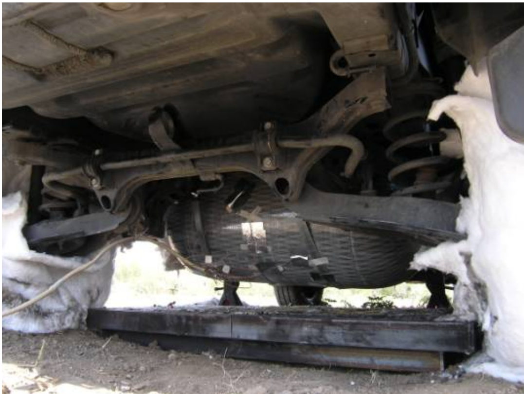
Figure B-2. Cylinder Mounted Under Vehicle, Bonfire Pan in Place.
