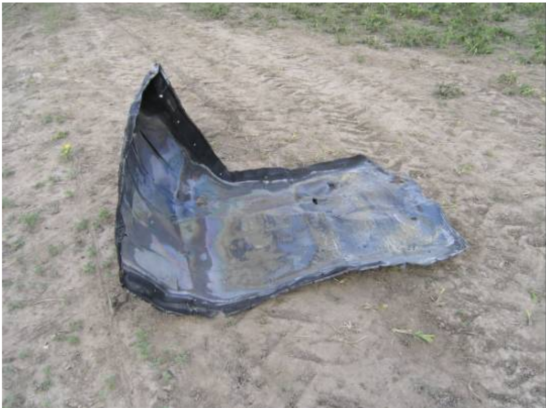
Figure B-12. Large Piece of Sheet Metal Found 112 ft From Test Site.
