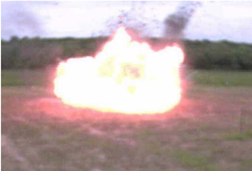
Figure 2. Hydrogen Tank Burst in FMVSS 304-Like Test
