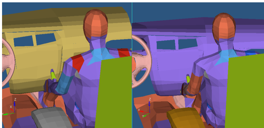
Figure 4. Comparison of Initial Hand Contact at t=60ms Between Crash Pulse Model (left) and Sled Test Model (right)
