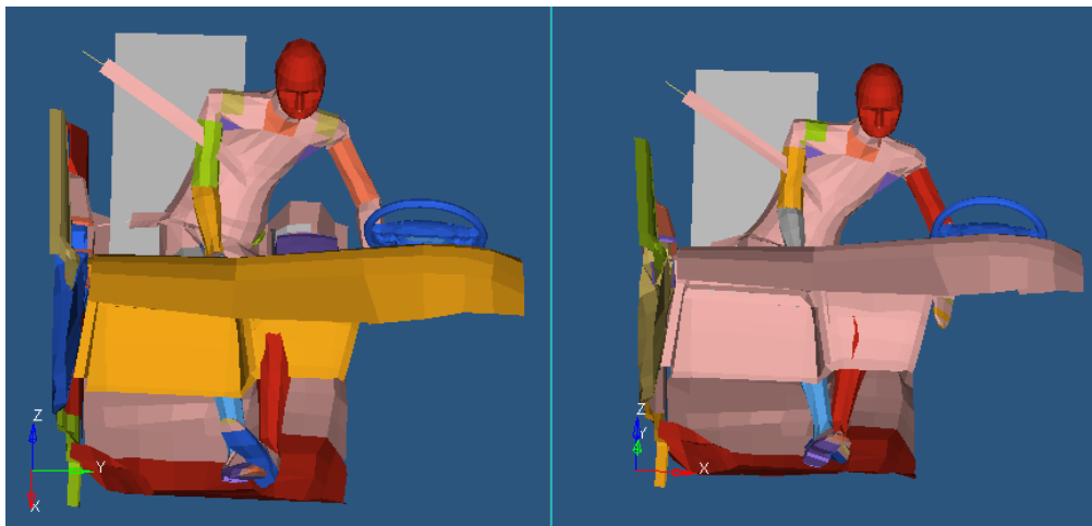
Figure 21. Rear View Comparison of Occupant Interaction with Center Console at t=90\text{ms} between 3-Point Belt Crash Pulse Model (left) and 3-Point Belt Sled Test Model (right)
