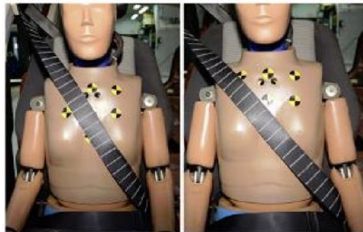
Figure 4. Sled tests of small female dummy, midtrack seat position: D-ring full-up (left), full-down (right)
