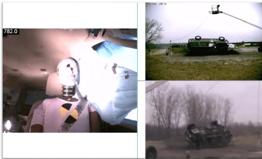
Figure 2. NHTSA Test No. 6960 Vehicle initial conditions contact (superimposed and synchronized video)
