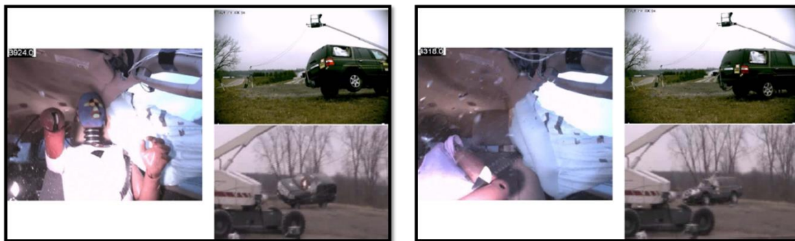
Figure 7. NHTSA Test No. 6960 8th quarter-turn left wheel contact the ground at 3924 and 4318 ms
