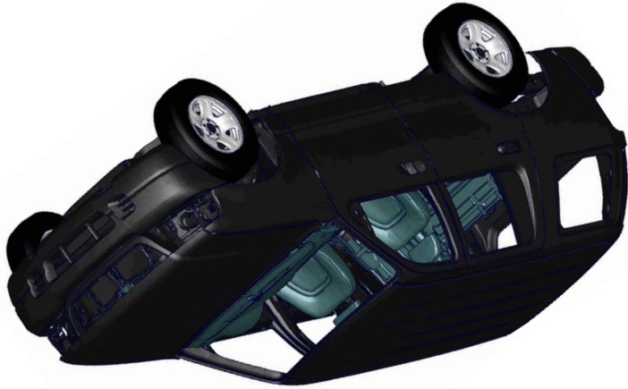
Vehicle model simulation with original roof crush characteristics without occupant
