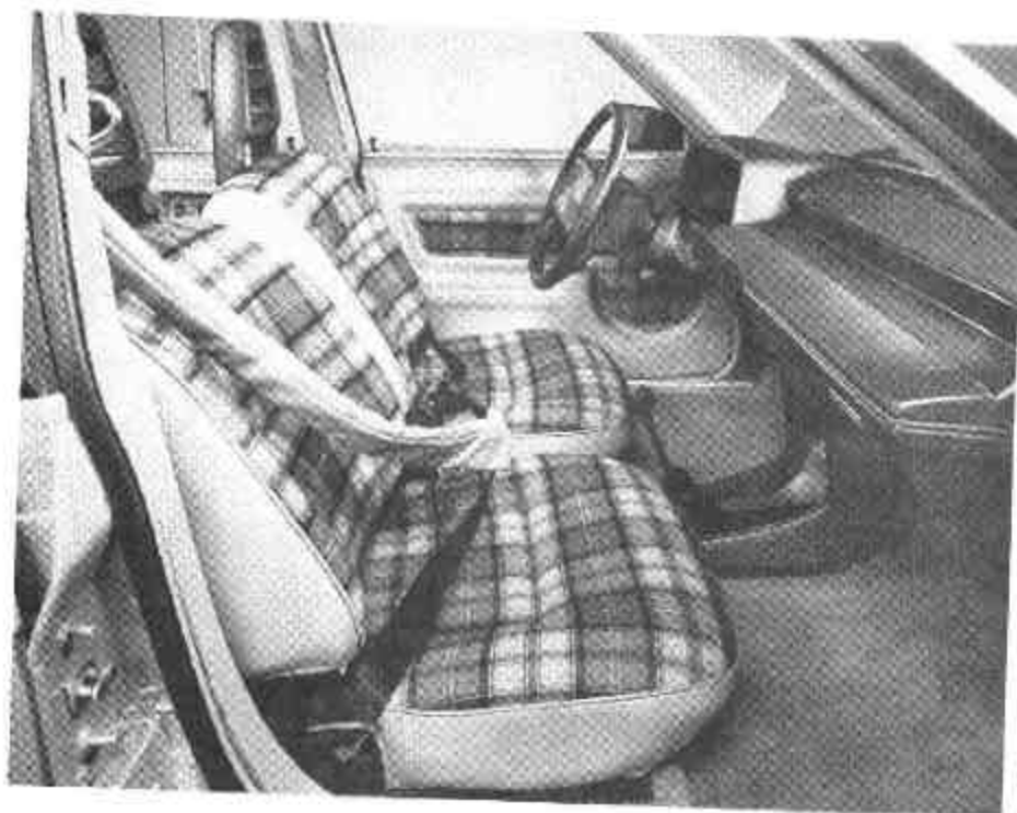
Figure 12. RSV Passenger Air Belt and Knee Blocker
