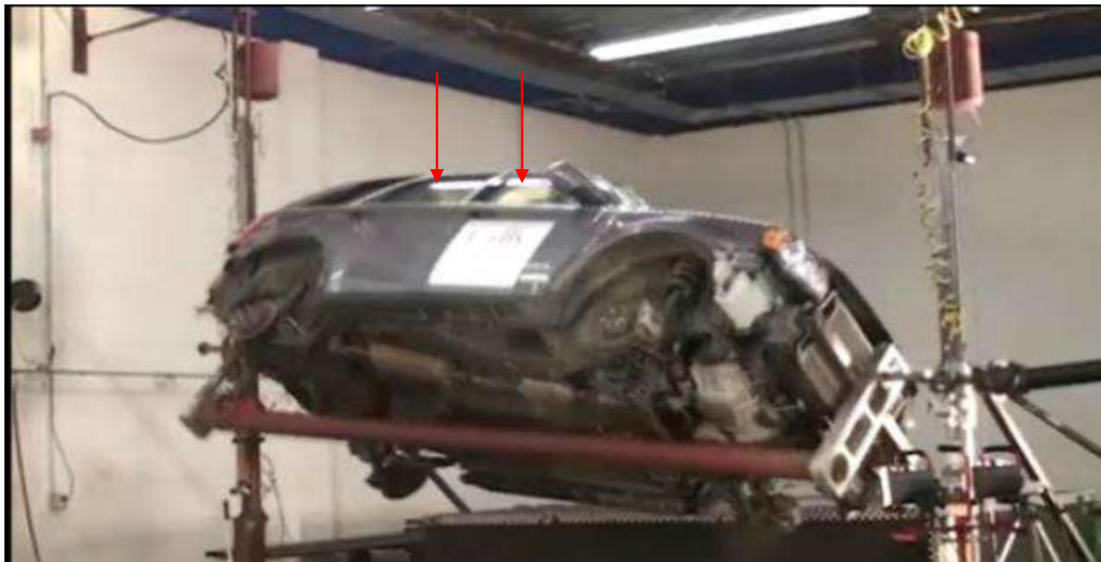
Figure 1. Photo Illustrating No Window Failures During Impact
