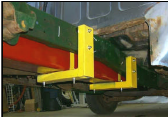
Figure 6: Centre and front tank brackets bolted to the frame rail.
