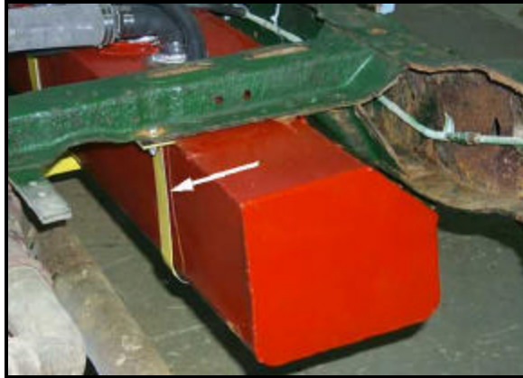
Figure 8: Rear tank strap (shown here with the truck box removed).
