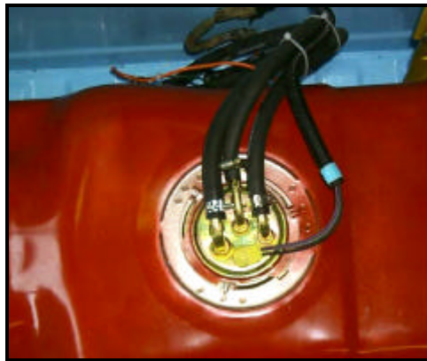
Figure 4: Fuel hose connections to the tank.
