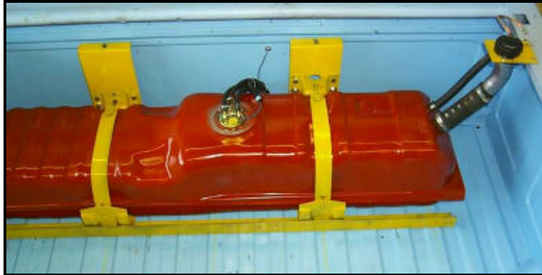
Figure 11: Bed tank secured in position.
