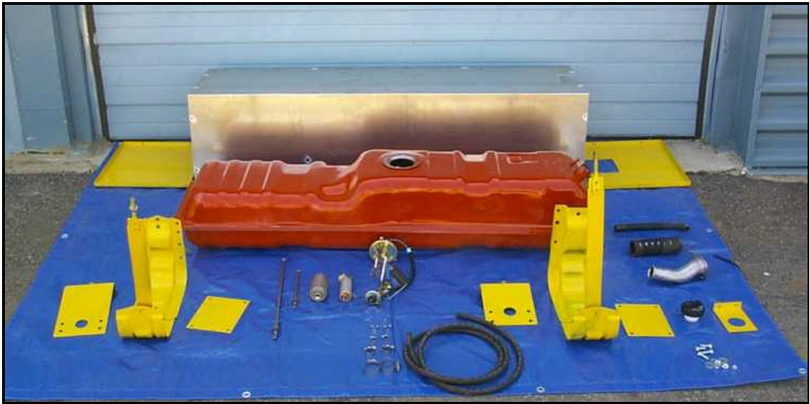
Figure 14: Major components of the box mounted tank system.
