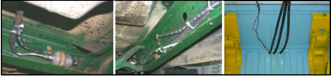
Figure 3: Typical routing of fuel hoses.
