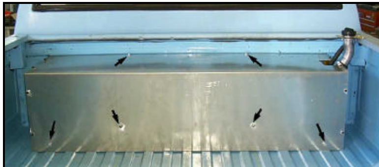
Figure 12: Fasten the tank cover. The bolt and nut locations are indicated.
