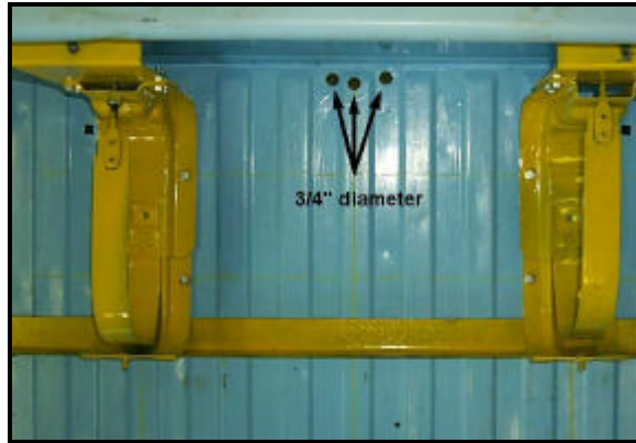
Figure 9: Three 3/4" holes drilled in the box floor.
