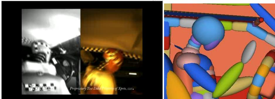
**Figure 8 - Side View Comparison Chrysler 300 JRS test and MADYMO Simulation**
