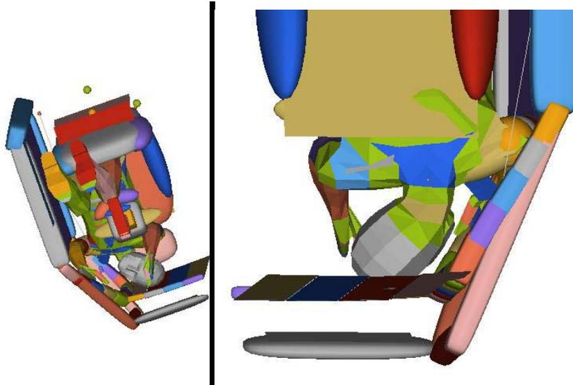
**Figure 12 – Frontal (left) and Back (right) view of Human Facet Model with roof intrusion.**
