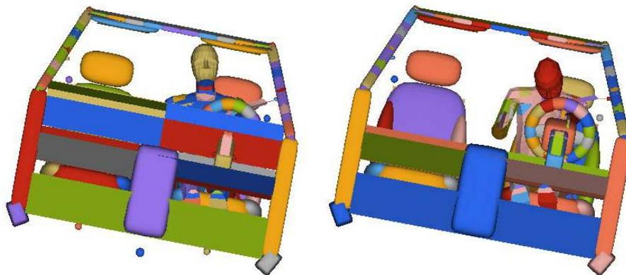
**Figure 9 - Frontal View of Human Facet Model Rollover Simulation with active muscle restraints (left) and without active muscle restraints (right)**
