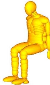
**Figure 3– TNO’s Hybrid III Ellipsoid Model (TNO Automotive-MM, 2005)**
