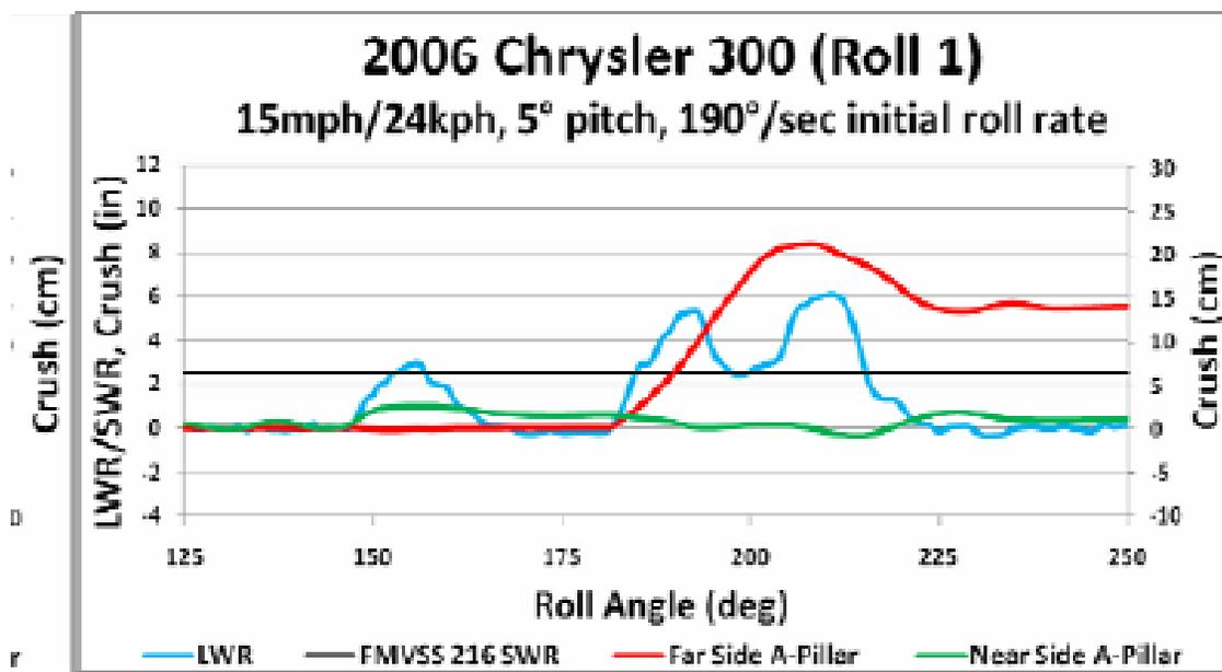
Figure 2- 2006 Chrysler 300 Roof Crush vs. Roll Angle (Friedman 2009)
