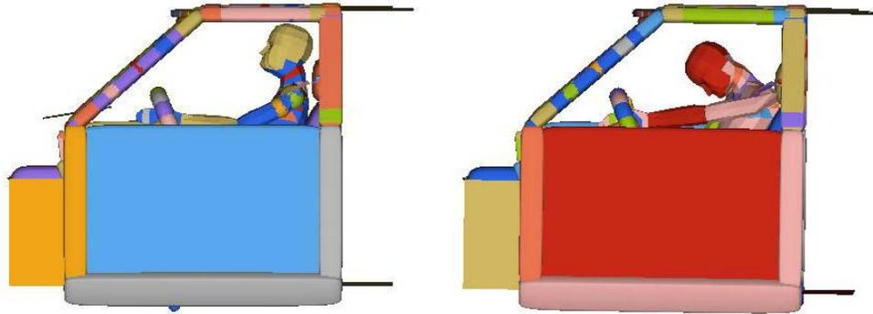
**Figure 10 - Side View of Human Facet Model Rollover Simulation with active muscle restraints (left) and without active muscle restraints (right)**
