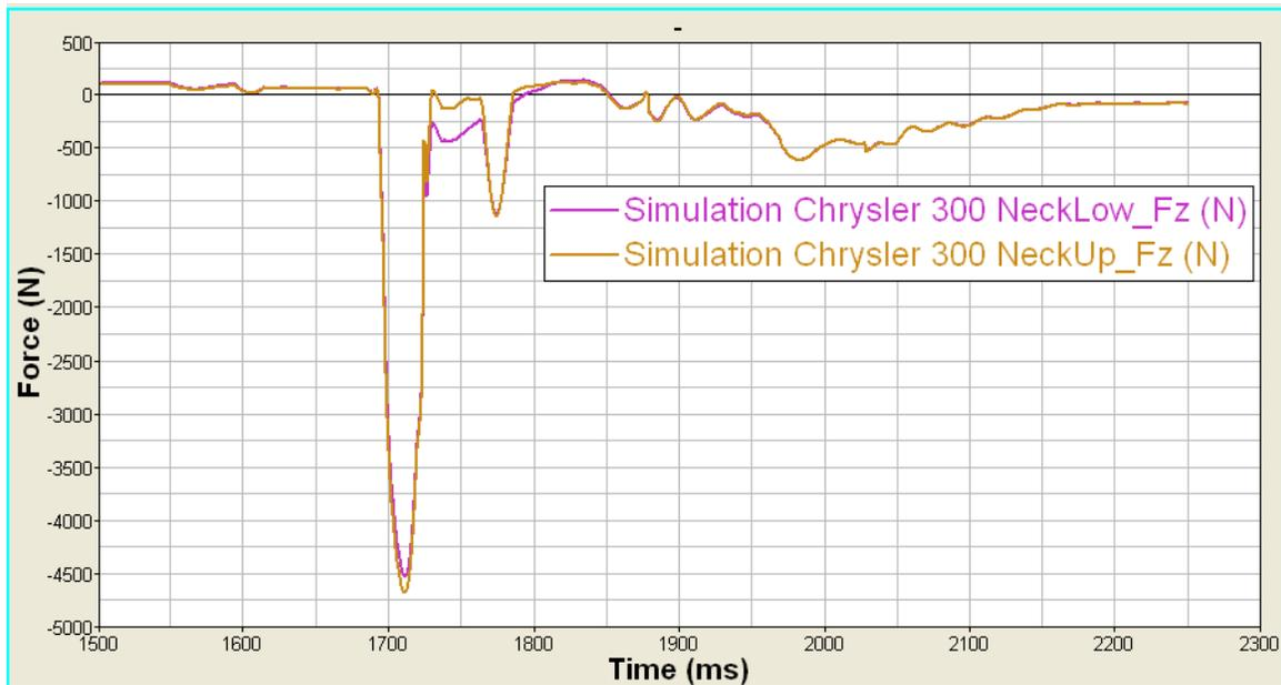
**Figure 5 -Hybrid III Simulation Compression Force**
