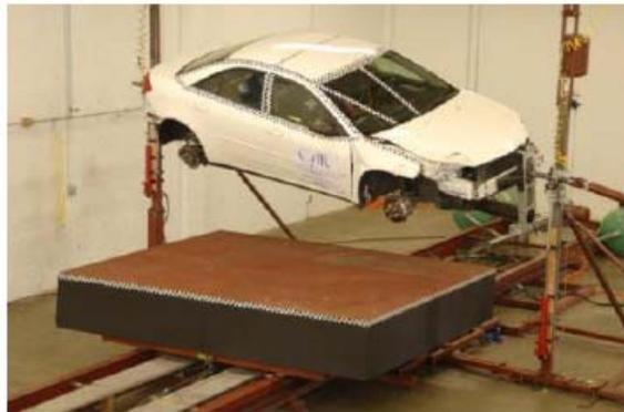
Figure 1 -JRS Test Fixture with mounted vehicle
