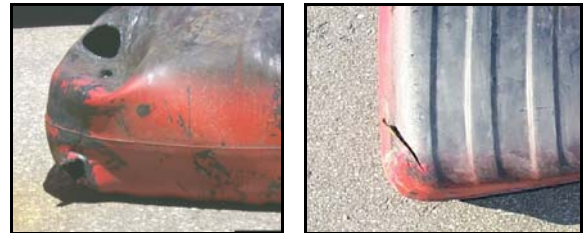
Figure 12. Puncture and slash damage to plastic tank
