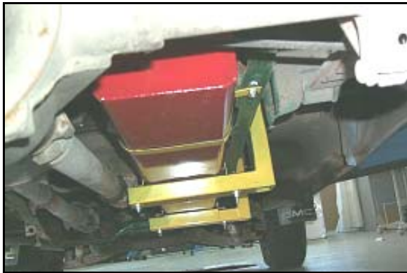
Figure 6. Typical center-mounted tank installation – Rear View
