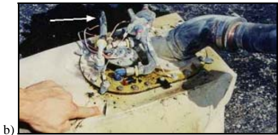
Figure 9. Steel housing for bladder [arrows show ruptured seam (a)]; cut in top of fuel cell [arrow shows sealed break-away fuel coupling (b)]
