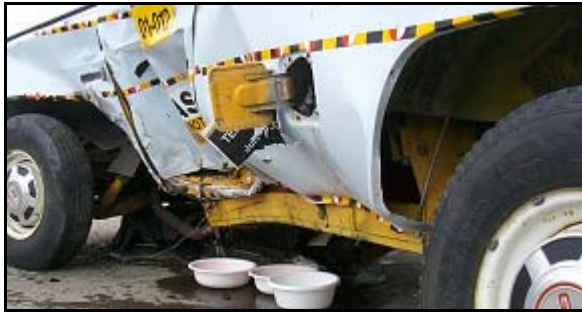
Figure 11. Damage to the modified tank protective frame
