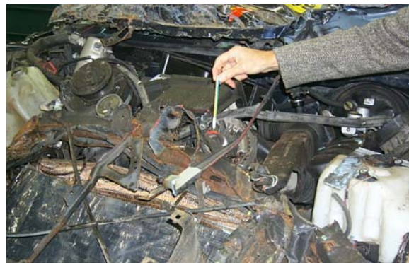
Figure 16. Caprice engine compartment after test showing hard points that contacted the fuel tank
