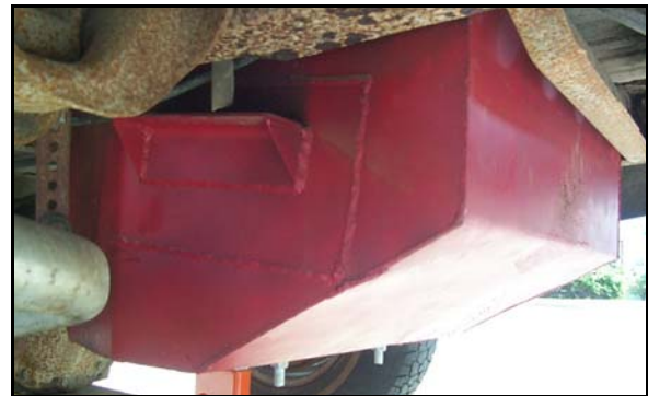
Figure 13. After market rear mounted tank
