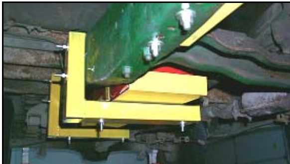
Figure 7. Typical center-mounted tank installation – Front View
