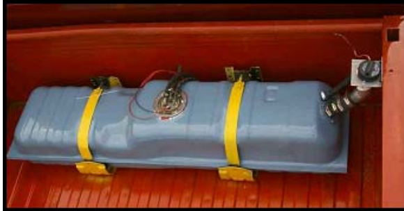
Figure 3. OEM bed tank installation with OEM brackets
