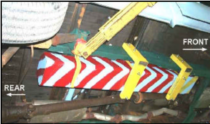
Figure 1: Typical center-mounted tank installation.
