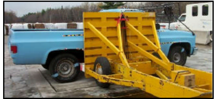
Figure 3: Alignment of the FMVSS 301 barrier for side collision.
