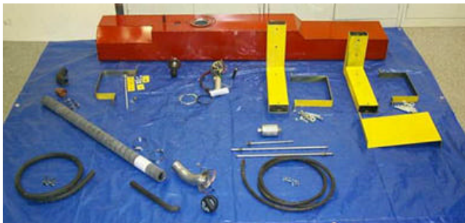
Figure 6: Center mounted tank and components
