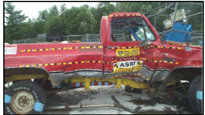
Figure 5: Typical pickup truck damage following a collision from a Caprice.
